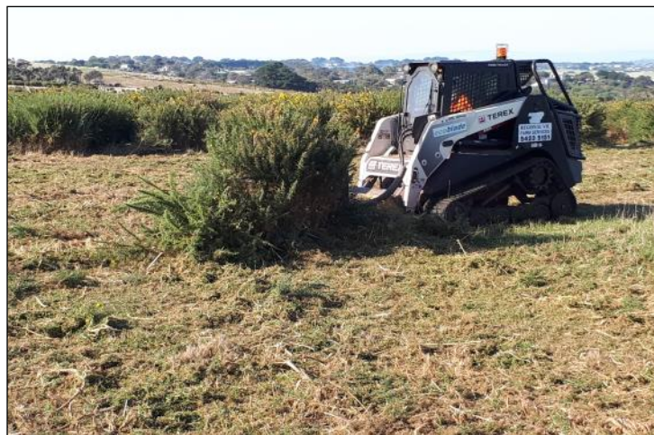
The EcoBlade in action cutting, painting and mulching gorse in one pass.
